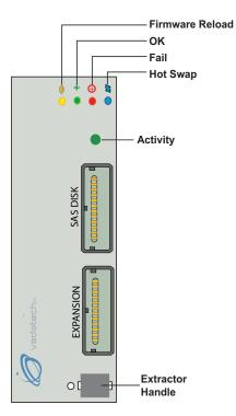
FIGURE 2. AMC606 Front Panel
