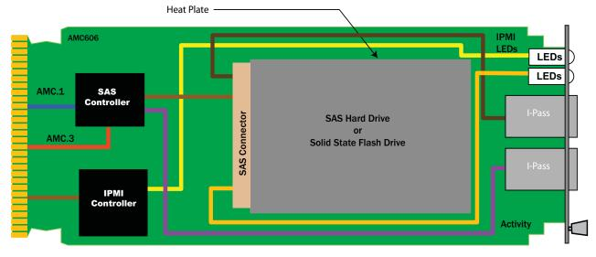
FIGURE 1. AMC606 Functional Block Diagram
